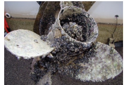
Invasive mussels attach to hard surfaces and are easily transportable by boats and equipment.
